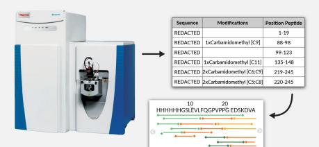
Step 3. Dithiothreitol (DTT) is used to reduce disulfide bonds before repeating the multiple enzyme digestion, nano-LC and high-resolution Orbitrap MS/MS analysis. This analysis accurately detects disulfide bonds within proteins and identifies the position of cysteins involved in the bridges.
